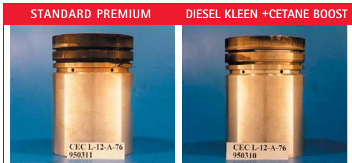
Comparison of piston cleanliness using a standard premium diesel fuel versus diesel fuel treated with Diesel Kleen +Cetane Boost.
